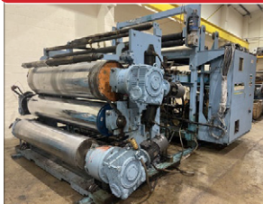
2290mm wide Davis Standard sheet extrusion line
