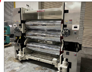
1650mm wide Welex 3 roll polishing stack
